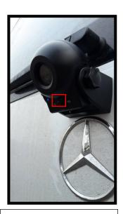
8. Mount the camera in the desired location on your vehicle using the magnet or adhesive Velcro (provided), and ensure that the device is switched ON by pressing the middle button (see red square) until the blue LED is lit.
